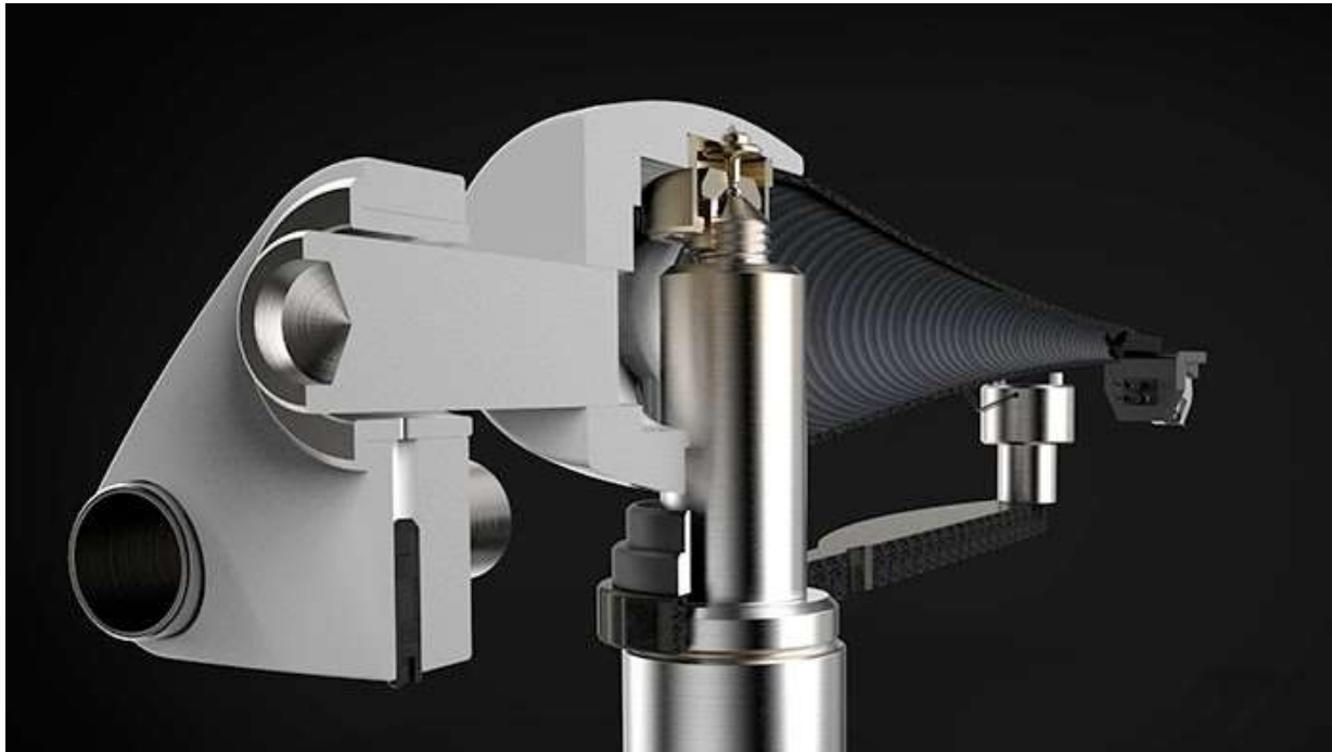
Kinematic Bearing: The A.C.T. 25 Tonearm Bearing in section
